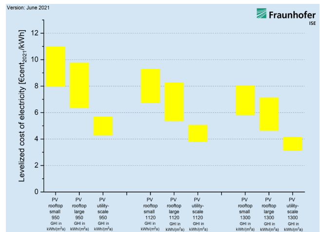
Figure 7: LCOE of PV systems in Germany based on system type and solar irradiation (GHI in kWh/(m 2 a)) in 2021.
